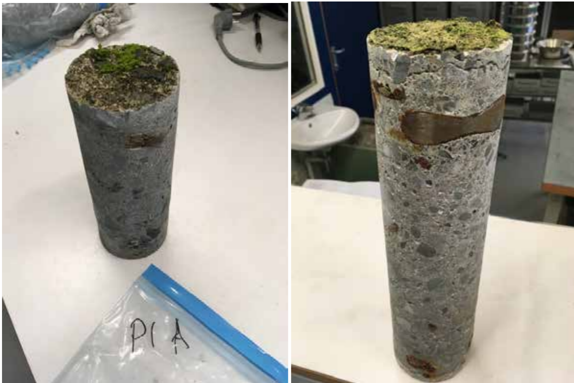
Sample 1A. Nice homogeneous concrete, well-proportioned. Minimal cracking, minimal damage. Good impression of sample.
