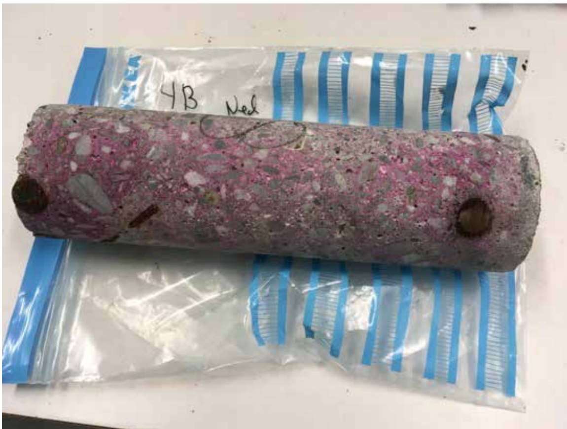
Sample 1A. Nice homogeneous concrete, well-proportioned. Minimal cracking, minimal damage. Good impression of sample.
