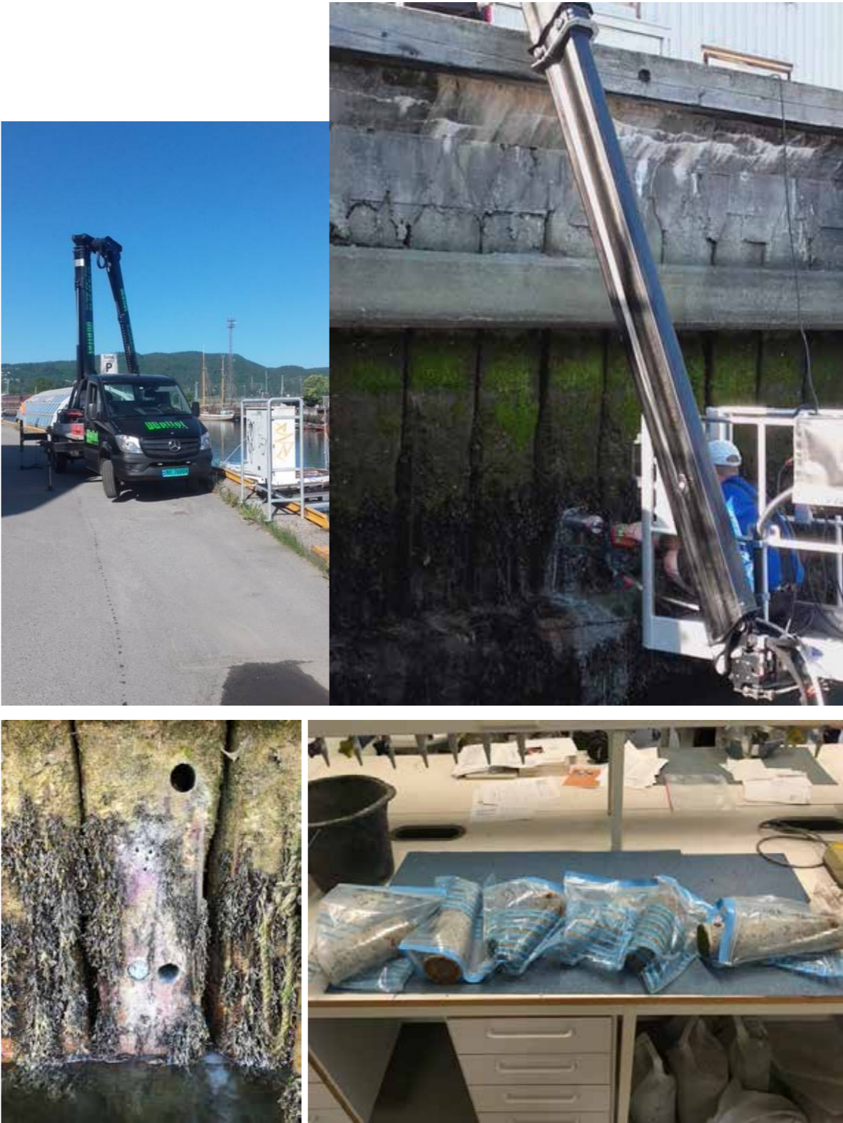
Concrete has good strength, and the corrosion of reinforcements inside the concrete is minor. The concrete surface is degraded, severely in some places, primarily due to external chemical weathering, as well as some frost damage.
